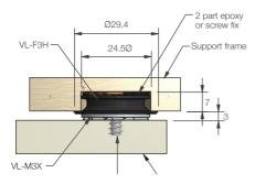
Through section showing surface mounted adhesive installation
