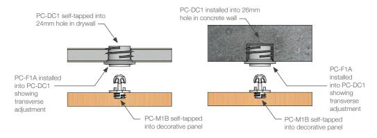
The Fastmount® multi-award winning system has revolutionized the mounting of panels. Panels can easily be removed and refitted in any sequence time after time. For further information or technical support contact: info@fastmount.com
