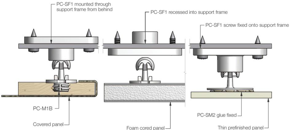
The Fastmount® multi-award winning system has revolutionized the mounting of panels. Panels can easily be removed and refitted in any sequence time after time. For further information or technical support contact: [info@fastmount.com](mailto:info@fastmount.com)
